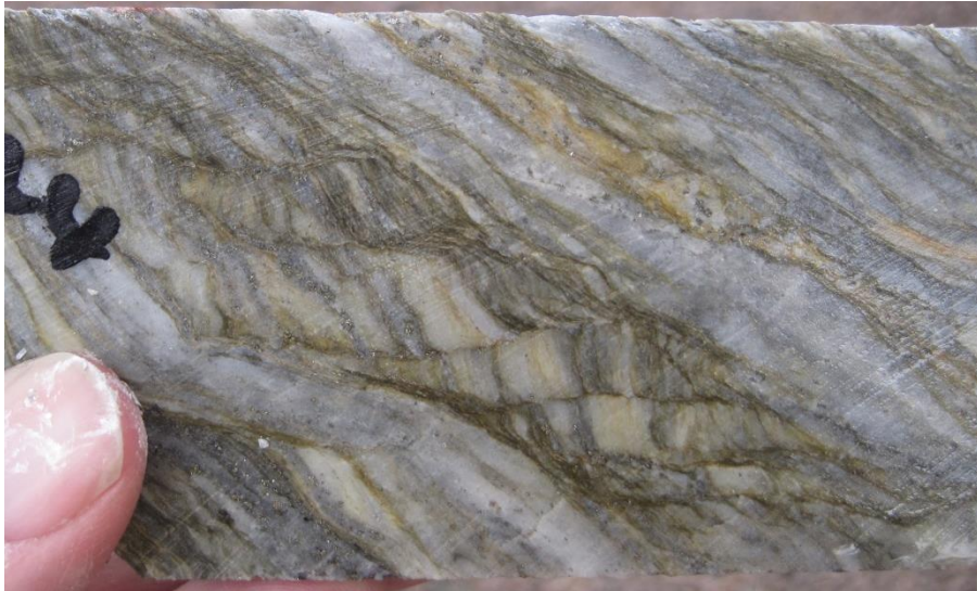
Figure 7-15: High-Grade Gold Mineralization from Silica Hill (WMD006)
