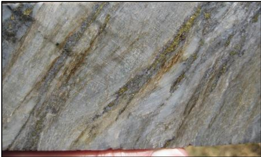
Figure 7.7 High-grade Gold Mineralization from Da Tambuk (ADD006, 56.7 g/t Gold and 1.60% Copper); Wispy Chalcopryite within a Silicified Sericite Schist
