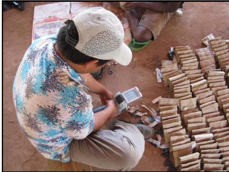
Plate 9. Niton X-ray analyzing shallow soil samples.
