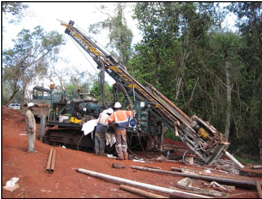
Plate 8. Drilling of a shallow inclined diamond hole, Magambazi North
