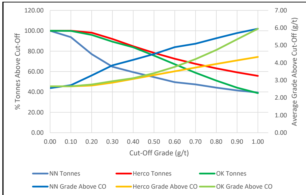
Figure 14.11 Grade-Tonnage Curve Comparison of OK Model with NN and DGM Models
